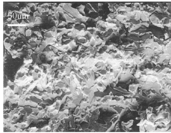
Figure 9 Fracture surface of Fe-49Co-2V alloy air-cooled from 820^\circ\text{C} .
